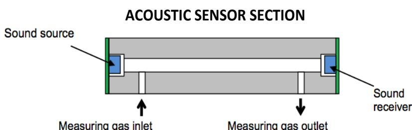
A schematic diagram of the sonic sensor is shown above. This sensor emits a sound from the sound source into a tube in which a measuring gas flows and then measures the time  $\tau$  in which the sound travels through the measuring gas and arrives at the sound receiver. The speed of sound that travels through the measuring gas v<sub>GAS</sub> can be expressed as the following formula:
