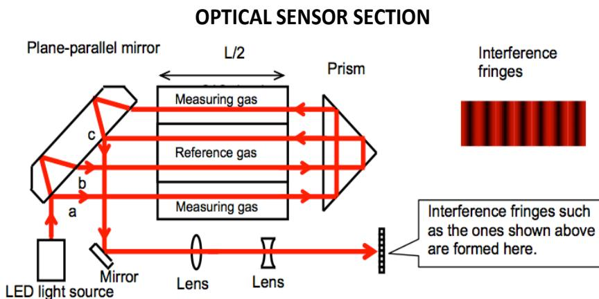
A schematic diagram of the interferometer used in the optical sensor is shown above. This interferometer forms "interference fringes" that move in proportion to the "differences of refractive index" between the measuring and reference gases. The movement distance of interference fringes  $\Delta\theta$  can be expressed as the following formula:
